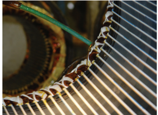
Figure 1.12.c - Resin applied by continuous flow process
