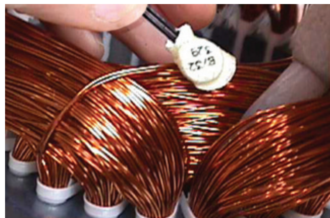
Figure 7.6 - Thermostat installation in the winding
